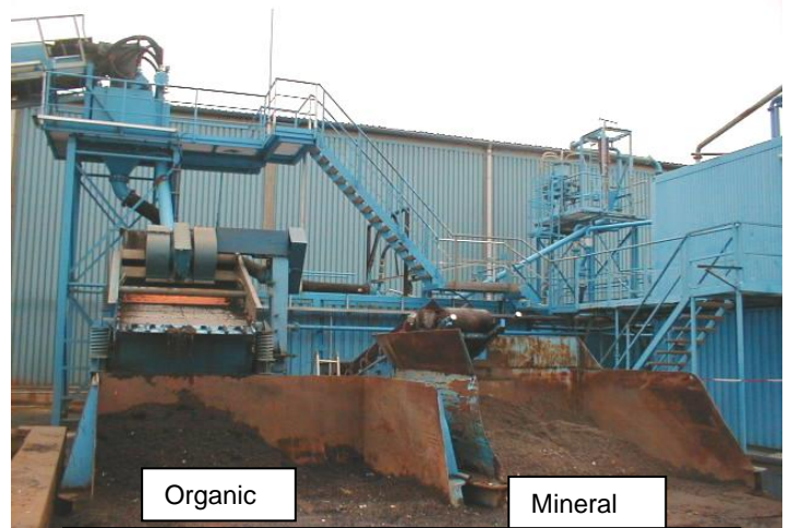
Hose Washer is the heart of the Soil Washing Plant
